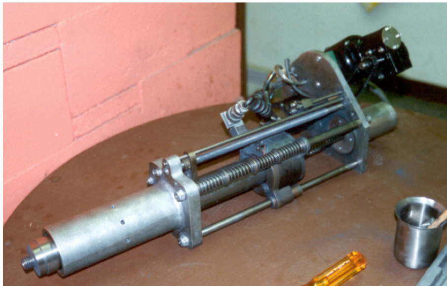
Figure 11. Photograph of the Control Element Drives
